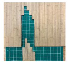
**Step 2**. Cut out the pattern from the flooring sheet. Use a combination of a sharp blade and scissors to cut along the laser lines.
